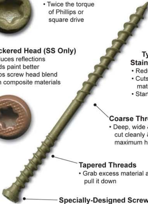
C-Deck Screw Specially-designed head and dual thread pull excess material into hole while countersinking
