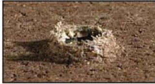
Standard Screw Causes 'mushrooming' of excess composite material
