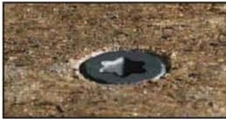
C-Deck Screw Specially-designed head and dual thread pull excess material into hole while countersinking
